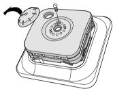
Then slide the control to the required position using a small screwdriver.
