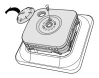
3. Connect power, voltage 230 VAC, load and floor sensor cable.
