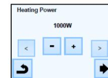
Press the (◀) or (▶) keys to select a unit, press the (+) or (-) keys to modify the heating power. This value is used to estimate the running cost of the system. You can return to the previous menu by pressing the ↶ key. Press the ▶ key in the bottom right corner to continue.
