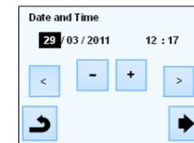
Select the time format 12H or 24H using the same method as above. Press the (◀) or (▶) keys to activate the value to be modified. Each time a value is highlighted, it can be modified by pressing the (+) or (-) keys. Press the ▶ key in the bottom right corner to continue to the next part of the installation. You can return to the previous menu by pressing the ↶ key.
