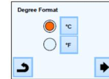
Select the degree format chosen by pressing on the touch button near the degrees. The active option is colored red. Press the ▶ key in the bottom right corner to continue to the next part of the installation. You can return to the previous menu by pressing the ↶ key.
