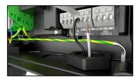
$\mbox{\bf Note:}$  When using a single thermistor, connect to terminal labelled TEMP1.
