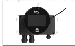
c. Remove the cover carefully. The board-to-board cable is connected by a zip tie at each end. Avoid straining the wire between the base and the cover.
