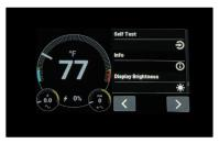
**Note:** If self-test is done without a load the unit will give circuit fault alarm.
