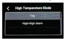
i. **High Temperature Trip** – Selecting this mode will make the circuit trip if any of the thermistor temperatures exceeds the High Temperature Trip setpoint (configured separately).
