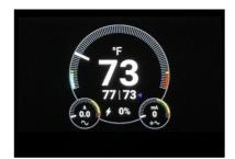
b) The small dials below indicate the circuit current (in A) and the ground current values (in mA). Both should be
