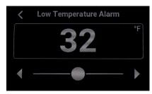
**Note:** When any sensor reading goes below this setpoint, this alarm will be triggered, and the Thermon logo will flash **BLUE.**
