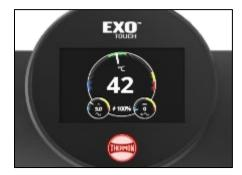
Once the boot up sequence has completed successfully, the circuit dial up will show up on the screen and the Thermon logo will turn Green. (within ~ 20 seconds).
