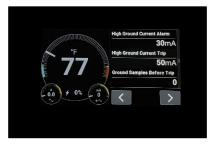
7.3.6.1. **High Ground Current Alarm** - The setpoint value range is 20 - 200 mA.
