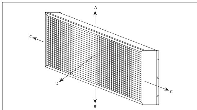
Figure 1 – Heater Clearance
